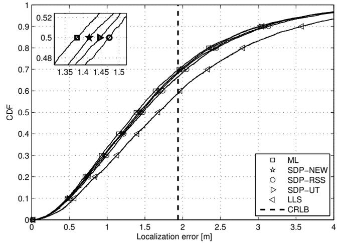
Fig. 1. The CDF of localization error for the compared estimators.  $\sigma_{dB} = 4$  dB,  $\rho = 0$  (uncorrelated case). The performance of the proposed SDP estimator is very close to the optimal ML estimator.
