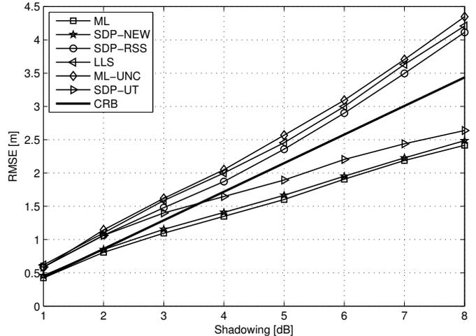
Fig. 3. The RMSE of the compared estimators versus the standard deviation of the shadowing with  $\rho = 0.8$ . As the shadowing increases, the difference between ML and ML-UNC increases.
