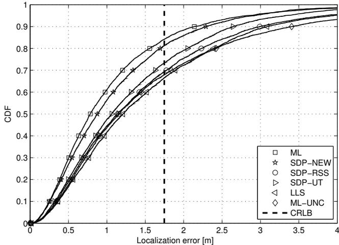
Fig. 2. The CDF of localization error for the compared estimators.  $\sigma_{dB} = 4$  dB,  $\rho = 0.8$  (correlated case). ML performs considerably better than ML-UNC meaning that using correlation among shadowing components can improve positioning accuracy considerably. The proposed SDP estimator is still close to ML and outperforms the other estimators.
